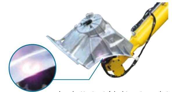
Laser heat treatment of shock tower-type product
